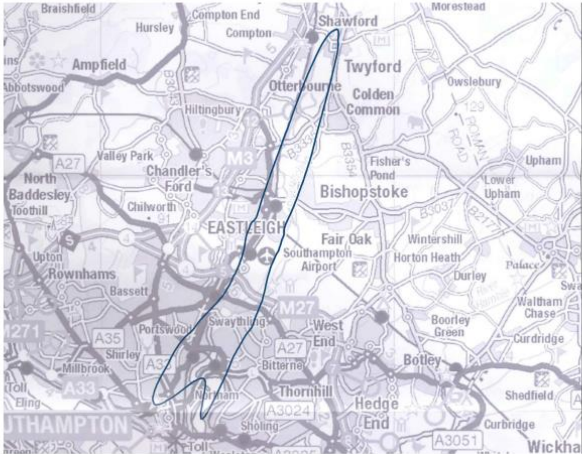
Figure 1-1: 2033 average summer day LA eq , 16hr contour with Runway Starter Extension as shown in s106
